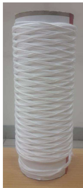
Figure 18 Winding product with a spiral leading structure, gear ratio u = \frac{1468}{179}
