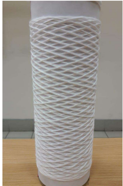
Figure 14 Winding product with a honeycomb structure, gear ratio u = \frac{68}{13}
