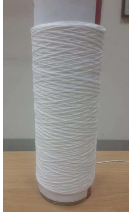
Figure 10 Winding product with a closed winding structure, gear ratio u = \frac{494}{61}
