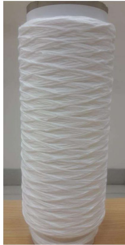
Figure 16 Winding product with a spiral structure, gear ratio u = \frac{992}{121}
