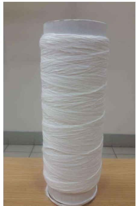
Figure 8 Winding product with a closed winding structure, gear ratio u = \frac{491}{49}
