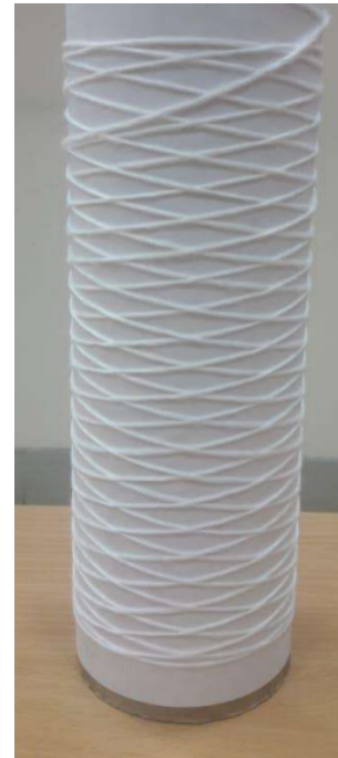
Figure 12 Winding product with a honeycomb structure, gear ratio u = \frac{46}{5}
